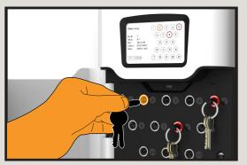
All keys and keysets are individually locked by the Traka 21 unit. Green LEDs indicate those keys to which this user has access. The user cannot remove keys highlighted by the Red LEDs which continue to remain locked in place.
